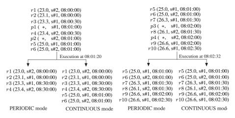
Figure 11: Tuples processed by the stream-to-cube operator in PERIODIC/CONTINUOUS mode
